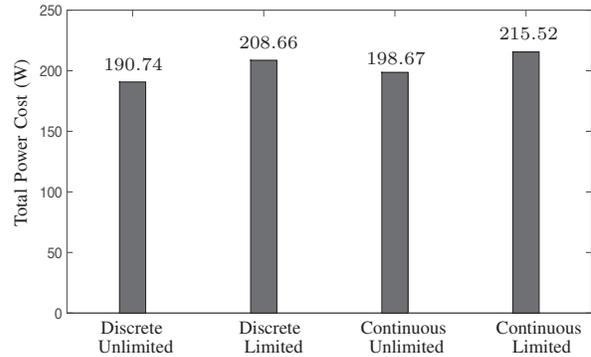
Figure 6. The total power cost of routing all demands by discrete and continuous programs under both limited and unlimited flow rule constraint
