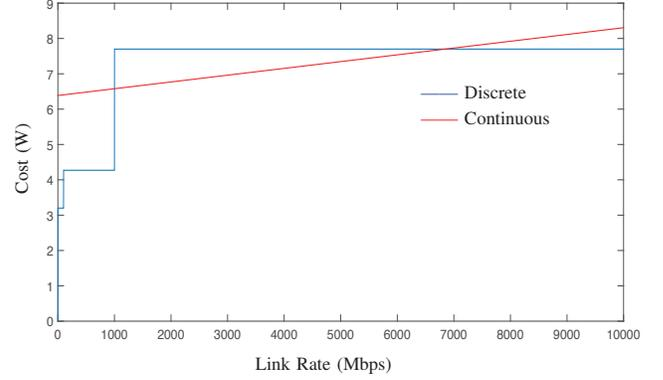
Figure 2. The discrete and continuous (curve fit) cost functions
